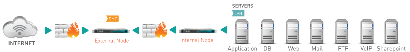
Figure 2 - Safe-T RSAccess Secure Front-end Solution Topology
